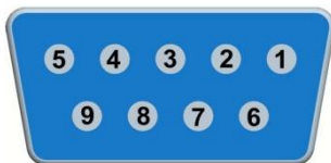
Figure 3-2 PDO-Profibus D-type connector pin out
